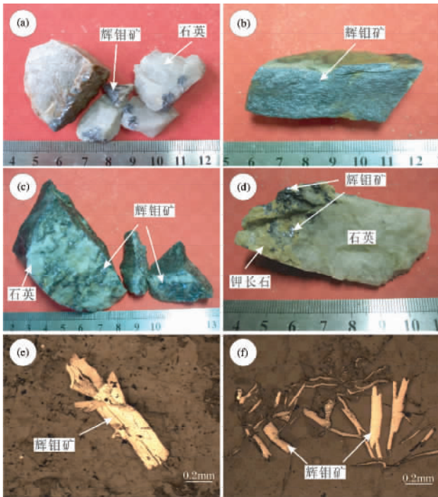
图4 东戈壁钼矿床矿石类型及辉钼矿特征 (a) -石英脉中的辉钼矿; (b) -围岩表面的薄膜状辉钼矿; (c) -浸染状辉钼矿; (d) -含辉钼矿的钾长石-石英脉; (e) -叶片状辉钼矿; (f) -鳞片状辉钼矿 Fig.4 Ore types and occurrence of molybdenite at Donggebi (a) -molybdenite aggregates in quartz vein; (b) -molybdenite film coating wallrock; (c) -disseminated molybdenite; (d) -molybdenite-bearing K-feldspar-quartz vein; (e) -molybdenite flakes in quartz vein; (f) -epidosome molybdenite
